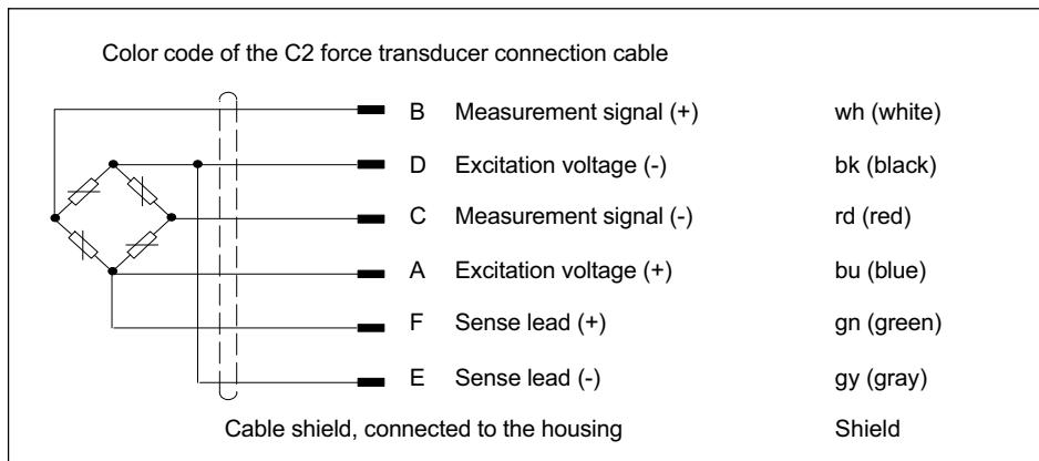
Fig. 8.1 Pin assignment in a 6-wire configuration
