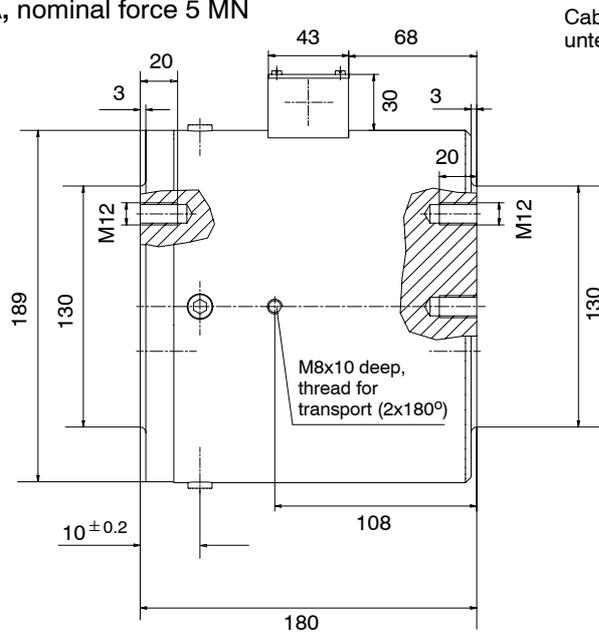
Cable:  $\varnothing 6.5$  mm; 6 m long, shielded, unterminated
