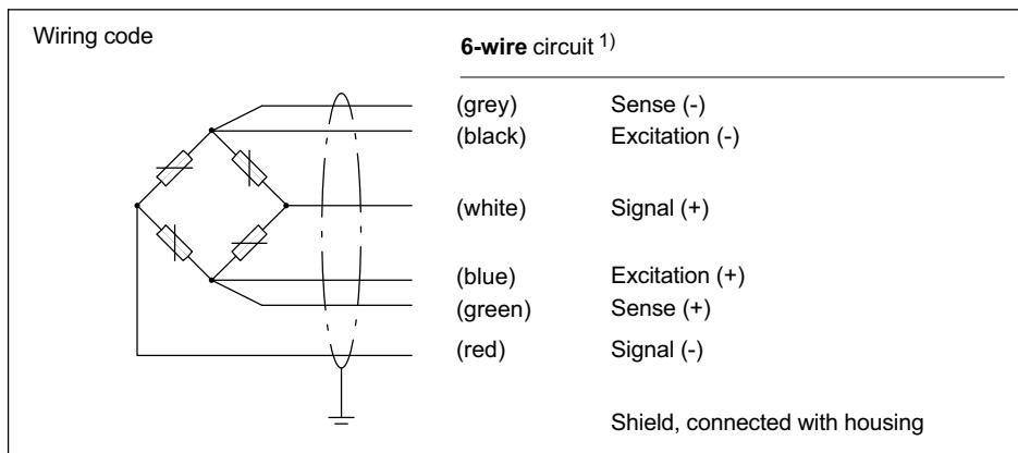
1) 1) When connecting to amplifiers in 4-wire technique you must connect the wires blue to green and black to gray. The following deviations occur with *unshortened* cables (3 m):
