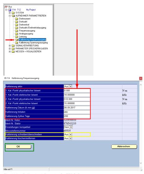
Fig. 14.2 Calibration information for TEDS, frequency output
