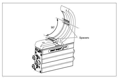
Fig. 8.16 Radial position of the spacers
