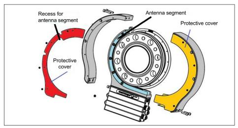
Fig. 8.8 Protective cover T12HP
