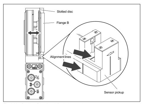
Fig. 8.21 Position of the slotted disc in the speed sensor
