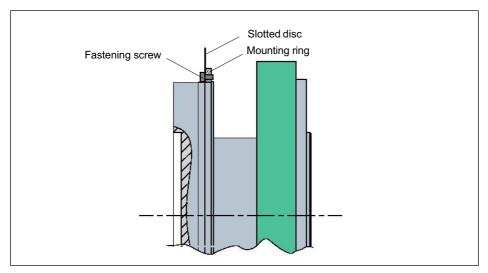
Fig. 8.1 Installing the slotted disc
