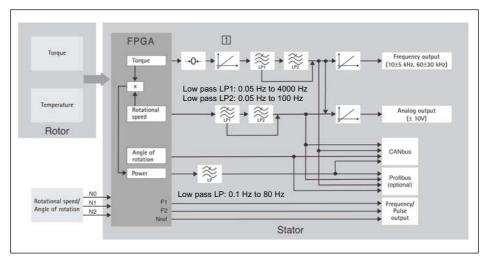
Fig. 6.1 Signal flow diagram
