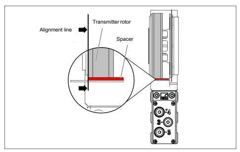
Fig. 8.18 Axial alignment to the rotor
