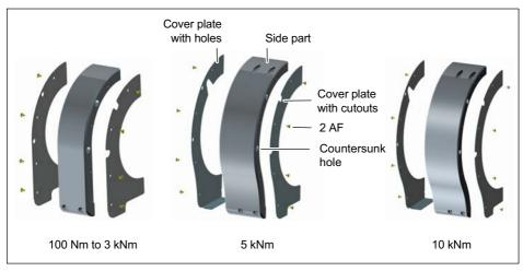
Fig. 8.7 Fitting the cover plates
