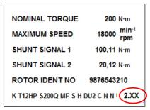
Fig. 23.3 Stator sticker: rotor hardware revision version
