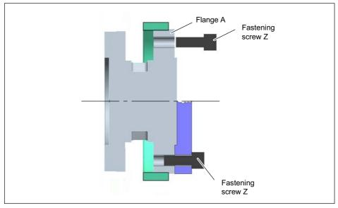
Fig. 8.3 Screw connections, flange A
