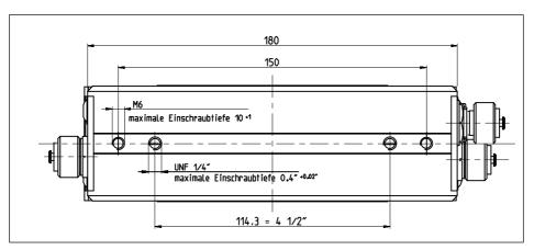
Fig. 8.12 Mounting holes in the stator housing (viewed from below)
