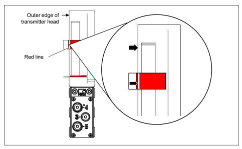
Fig. 8.17 Axial position of the spacers
