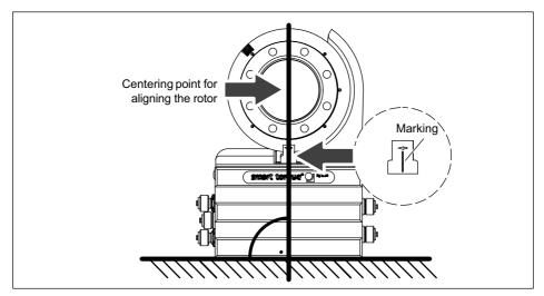
Fig. 8.22 Alignment markings on rotor and stator
