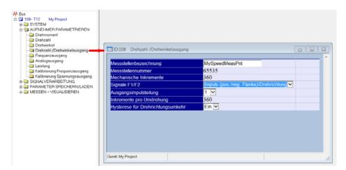
Under signal editing, only the measuring range as shown in figure ...(red) can be used in combination with TEDS functionality for TEDS angle of rotation. This means that the angle of rotation can only be measured with TEDS with the following setting.
