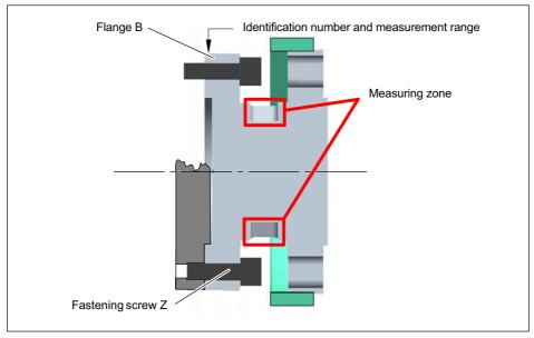
Fig. 8.2 Screw connections, flange B
