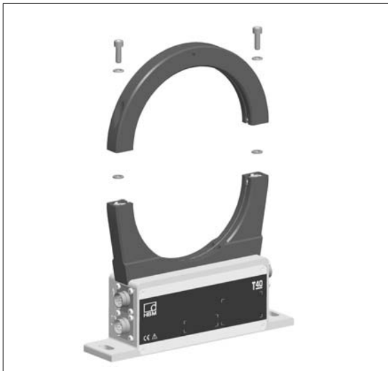
3. Dismantle antenna segment
