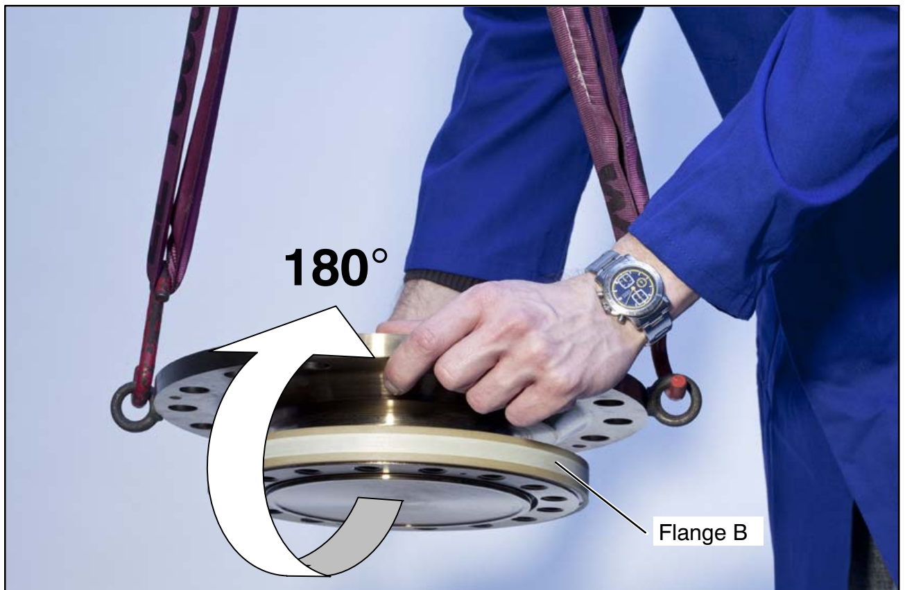
Fig. 4.2: Rotating the rotor
