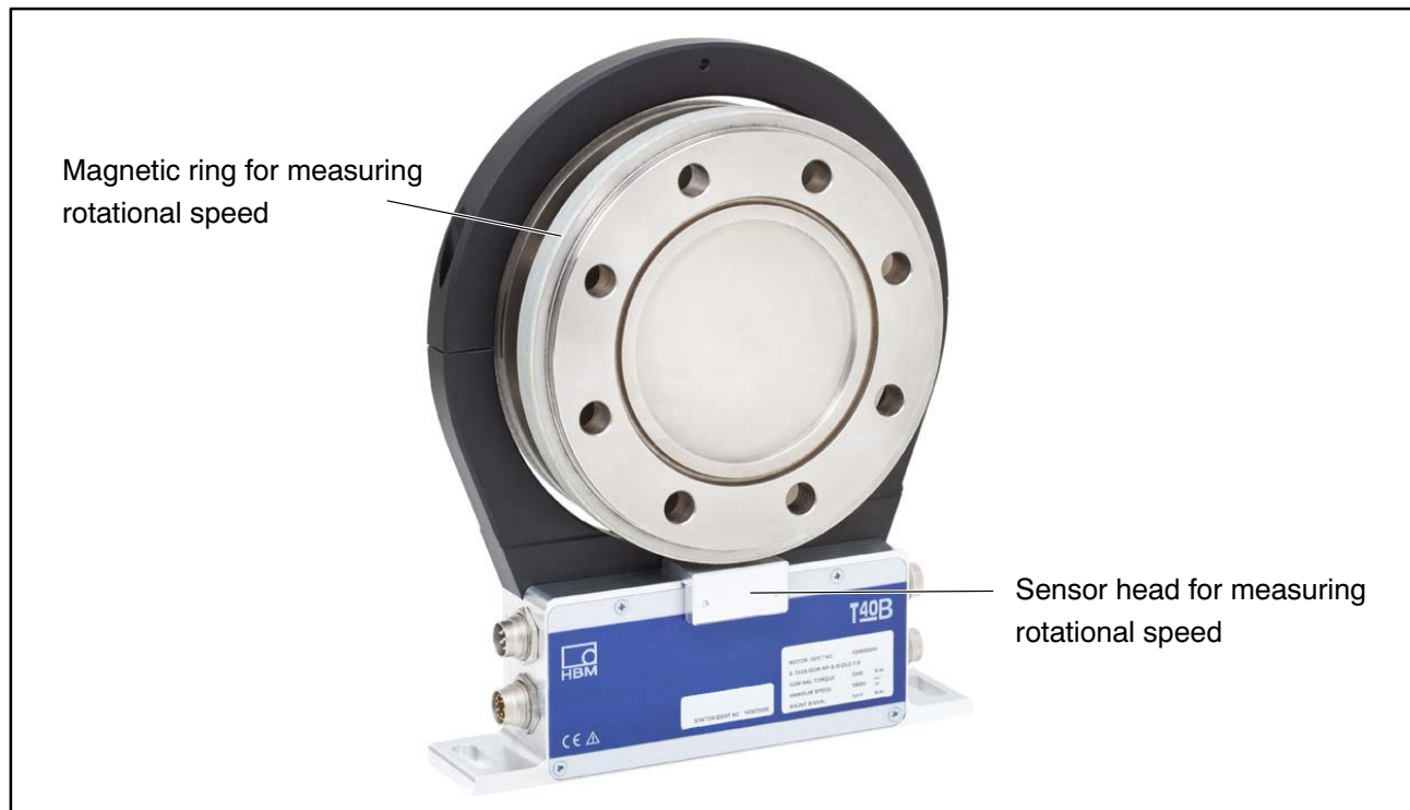
Fig. 4.7: Torque transducer with rotational speed measurement
