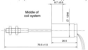
Plunger in mid position (auxiliary quantity for core assembly, zero balancing see Operating manual)
