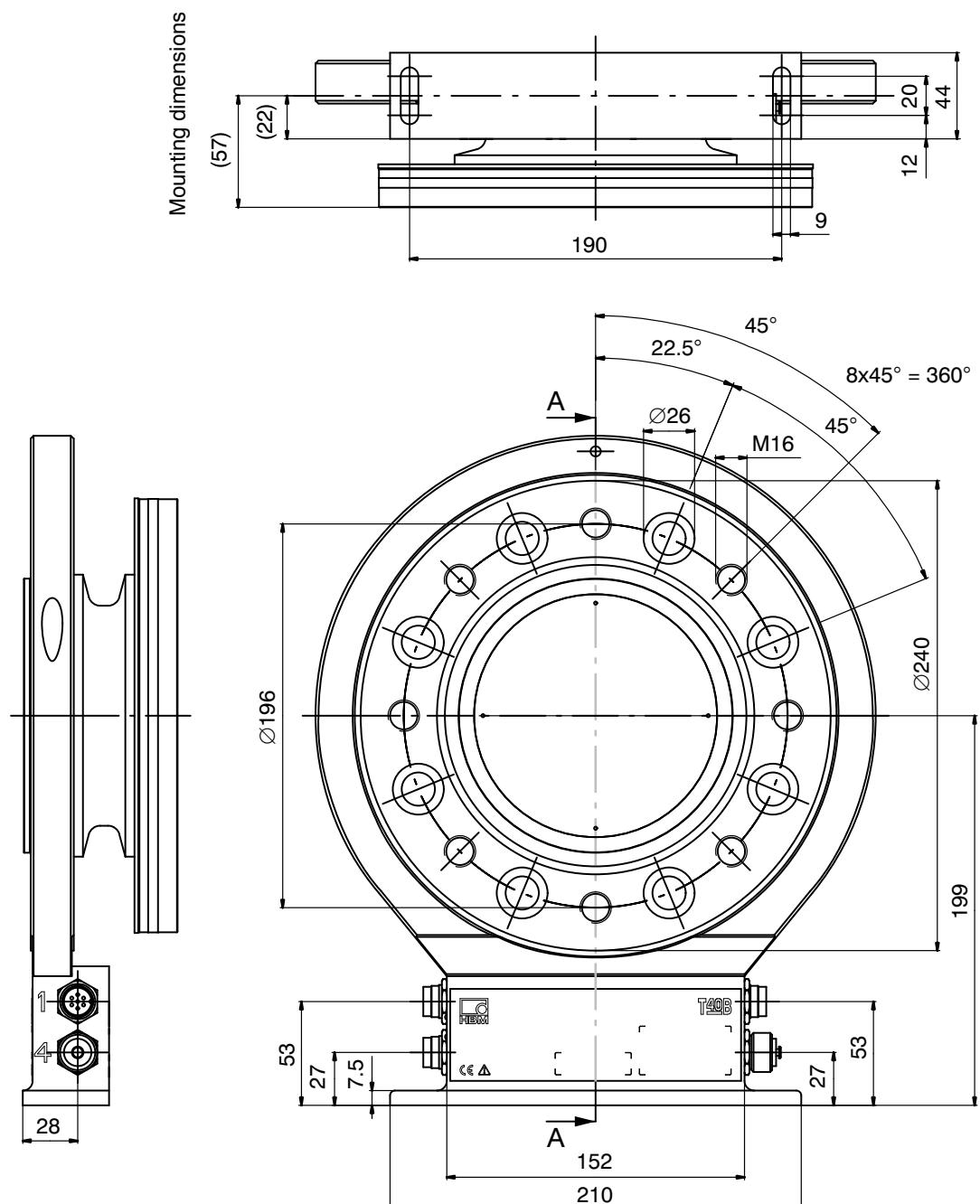
**Dimensions of T40B/10 kNm without rotational speed measurement, continued**
