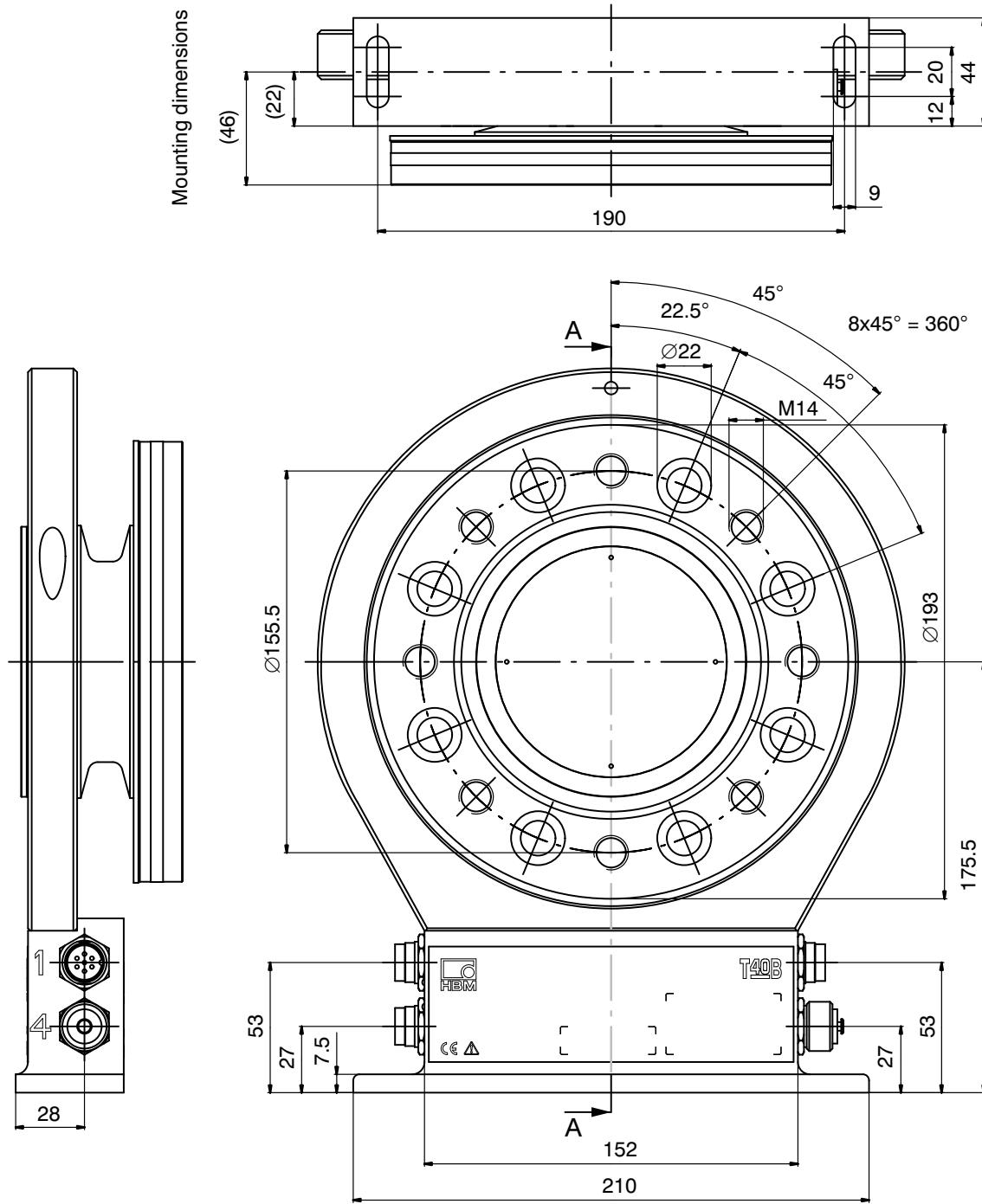
**Dimensions of T40B/5 kNm without rotational speed measurement, continued**
