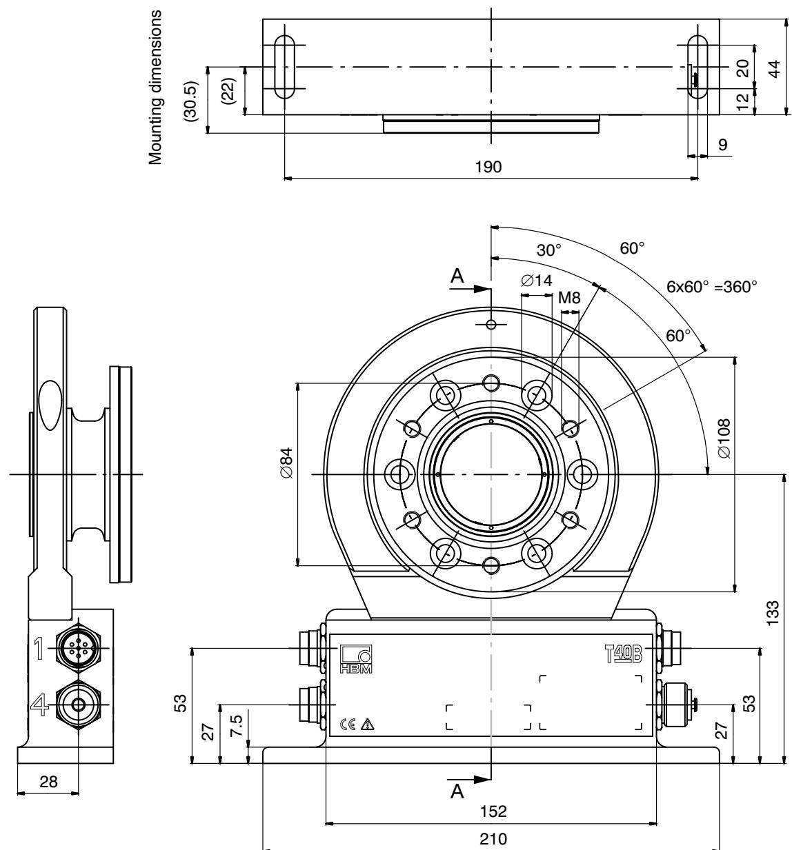
**Dimensions of T40B/200 Nm without rotational speed measurement, continued**
