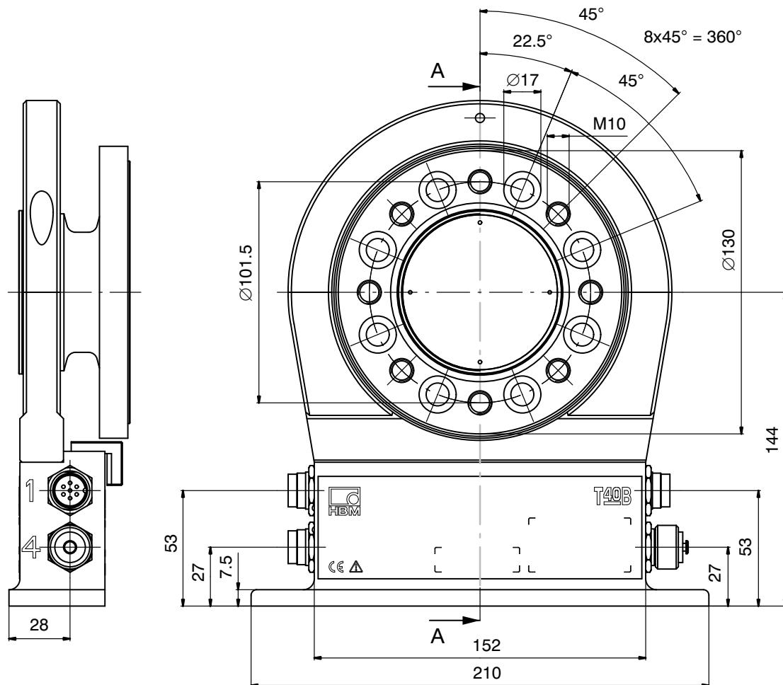
**Dimensions of T40B/500 Nm and 1 kNm with rotational speed measurement, continued**
